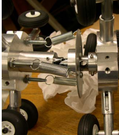
Fig. 3-7. Articulation, featuring universal joint and stiffening springs.
